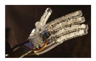
The Virginia Tech College of Engineering's Robotics and Mechanisms Laboratory created an improved fully articulated robotic hand. RAPHaEL 2 can firmly hold objects ranging from a soup can to a raw egg. It uses force and position feedback to automatically control the grasping force and finger position. Credit: Virginia Tech Photo
