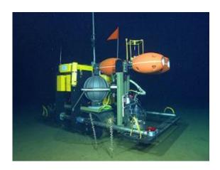
The Benthic Rover makes its way across the deep seafloor during a trial run in 2007. The "brains" of the vehicle are protected by a spherical titanium pressure housing. The orange and yellow objects are made of incompressible foam, whose buoyancy makes the Rover light enough underwater so that it won't sink into the soft deep-sea mud. Image: © 2007 MBARI
