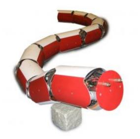
Anna Konda has 20 hydraulic motors that actuate the joints in its 75 kg body.
