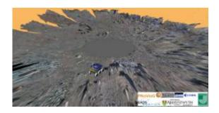
This is a frame from an animation generated from 33 stereo image pairs taken at the CNES SEROM Marsyard in Toulouse. Processing was performed using the ExoMars PanCam 3D Vision Software by Joanneum Research, Graz, Austria. The camera equipment (PanCam Analogue Camera - PAC) was provided by Aberystwyth University, UK (Prof. Dave Barnes). The images were acquired by ESA (Luc Joudrier). The ExoMars Rover model (status: Early 2008) was compiled by EADS Astrium Space, Stevenage, UK.
