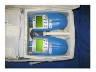
After space shuttle Discovery launched on Aug. 28, it delivered to the International Space Station a water quality monitoring kit developed by University of Utah chemists. Part of the kit, which is the size of a small ice chest, is shown here, with two commercially available color sensors that will be used during six months of testing to check for levels of the disinfectants iodine and silver in space station drinking water. Credit: NASA
