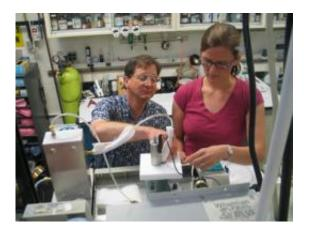
NIST research chemist Tom Bruno and postdoctoral researcher Tara Lovestead assemble an apparatus for detecting and measuring explosives and toxins. The sample is inside the blue column (lower center). Bruno enhanced the technique, called headspace analysis, to make it suitable for detecting low concentrations of polar, low-volatility compounds. Credit: Burrus/NIST
