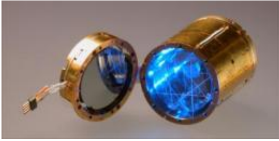
This is the BGO scintillator crystal (right, blue) and germanium disc (left). Credit: IAS / SINC
