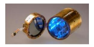
This is the BGO scintillator crystal (right, blue) and germanium disc (left). Credit: IAS / SINC
