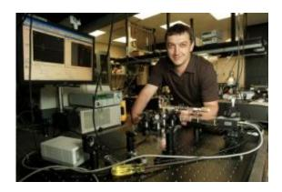
Gerard Wysocki, an electrical engineer at Princeton, worked with colleagues at Rice University to develop a highly portable and sensitive method for detecting nitric oxide gas, a key player in pollution and human physiology. The device uses a laser and an innovative type of polarizing filter to detect very small quantities of the gas. (Photo: Frank Wojciechowski)
