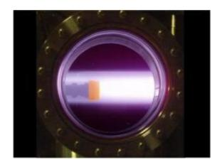
A hot (1,000C) tungsten sample is exposed to high-power deuterium plasma in the PISCES-B device to investigate plasma-surface interactions. Such research and experiments are conducted at the UCSD Center for Energy Research's PISCES lab, which is used to perform fundamental and experimental research in the field of boundary plasma science for fusion applications. Credit: UC San Diego
