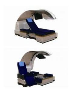
A bed-shaped robot which can transform from a bed (top) to a wheel chair (bottom). Japan's Panasonic Corp. has developed a "Robotic Bed" that can transform into a wheelchair to make life easier for elderly and disabled people, it announced
