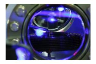
This is a view into the ultrahigh vacuum chamber in which strontium atoms are cooled and stored. In the upper third of the window, the blue fluorescent light of a cloud of cold strontium atoms (Sr) is to be seen. Credit: (Image: PTB)
