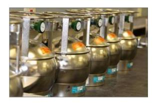
Storage canisters lined up in NREL's lab hold gas emission from cars that got a taste of higher levels of ethanol in the gasoline. Study results so far have shown that as ethanol increased, tailpipe emissions stayed largely the same. Credit: Heather Lammers
