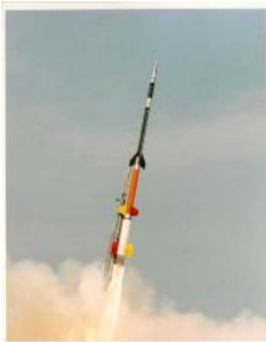
Black Brant XII suborbital sounding rocket. Photo Credit: NASA
