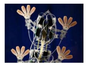
Stickybot has specially designed footpads, inspired by the surface of a gecko's foot, that allow it to climb smooth surfaces. MIT Assistant Professor Sangbae Kim worked on the robot as a graduate student at Stanford. Courtesy Sangbae Kim
