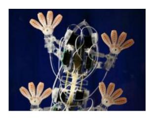
Stickybot has specially designed footpads, inspired by the surface of a gecko's foot, that allow it to climb smooth surfaces. MIT Assistant Professor Sangbae Kim worked on the robot as a graduate student at Stanford. Courtesy Sangbae Kim
