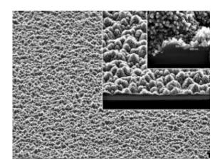
Chemical engineers at Oregon State University are using extraordinarily small films at the nanostructure level to improve the performance of eyeglasses and, ultimately, solar energy devices. These films, which resemble millions of tiny pyramids, reduce the reflectance of any light that strikes the material. (Image by Seung-Yeol Han)
