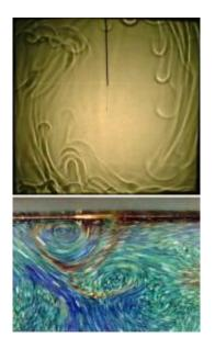
On the top is a shadowgraph visualization of rising and falling plumes in a turbulent fluid. On the bottom are small liquid-crystal spheres show the temperature and velocity in a fluid simultaneously. Credit: Top image: X. D. Shang, X. L. Qiu, P. Tong, and K.-Q. Xia, Phys. Rev. Lett. 90, 074501 (2003); Bottom image Y. B. Du and P. Tong, J. Fluid Mech. 407, 57 (2000).
