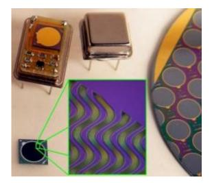
The microstructured semiconductor neutron detector is a portable device designed to detect neutrons, a signature radiation emitted by some nuclear materials used in nuclear weapons. Kansas State University's Douglas McGregor, professor of mechanical and nuclear engineering, and his team of researchers designed and developed the detector that was given a 2009 R&D 100 Award. Credit: K-State media relations
