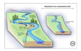
By reverse-engineering a meandering stream, researchers have shown two ingredients to be very important: vegetation to reinforce banks and prevent erosion, and sand to build point bars and block off cut-off channels and chutes. This knowledge will help stream restoration efforts in the future. Credit: Zina Deretsky, National Science Foundation
