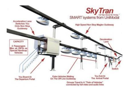
A passenger would enter a pod, type in where he or she wants to go, and the computer system would do the navigating (and driving). The pods would carry up to three people and travel up to 150 mph. The system would be computerized to deploy the pods to crowded areas, and smart enough to re-route to avoid traffic jams.
