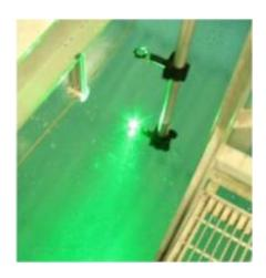
Scattered light from a 532 nm laser pulse can be seen as it enters the water in the Salt Water Tank Facility, and ionizes a small volume of water for acoustic generation. Air bubblers and controlled water and air temperatures can create ocean-like conditions in the laboratory. Credit: Naval Research Laboratory photo
