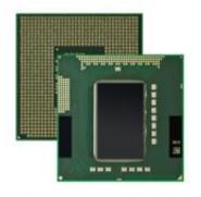
New Intel Core i7 mobile processors which include two-channel DDR3 1333 MHz memory support and full 1 x16 or 2 x8 PCI Express 2.0 graphics.
