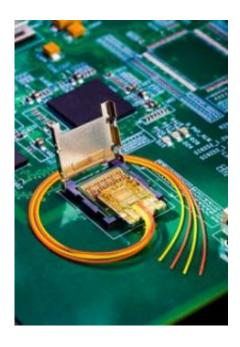
Light Peak module with 4 fibers. Each fiber capable of carrying data at 10 gigabits per second. Credit: Intel
