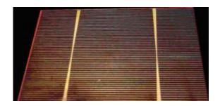
IMEC's i-PERC cell with shallow emitter and Cu metallization.
