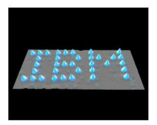
On this day in 1989, IBM Fellow Don Eigler became the first person in history to move and control an individual atom. Shortly thereafter, on November 11 of that year, Eigler and his team used a custom-built microscope to spell out the letters IBM with 35 xenon atoms.
