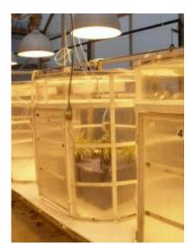
Experimental chambers in a Penn State University greenhouse were equipped with a charcoal filtration air supply system to measure ozone depletion rates. Credit: Photo by Dennis Decoteau
