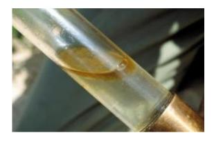
This is a transparent borehole sampling tube (bailer) showing layer of fuel oil floating on top of groundwater. Credit: Willem van Aken
