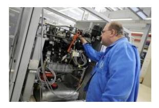
A technician of German automaker Volkswagen's adjusts a mini gas-fired power plant at the VW plant in the northern German city of Salzgitter. An ambitious project was unveiled in Germany on Wednesday to install mini gas-fired power plants in people's basements and produce as much electricity as two nuclear reactors within a year.
