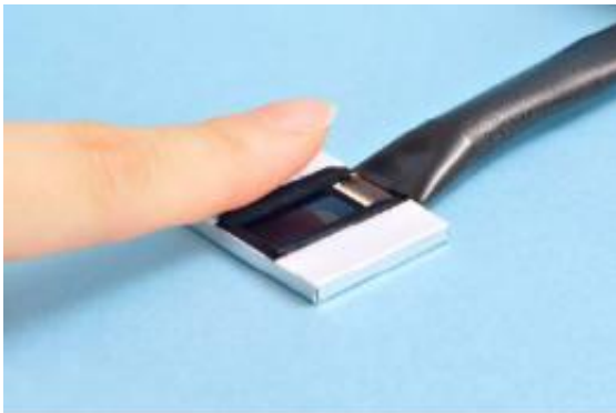
3mm thick finger vein authentication module (prototype unit)
