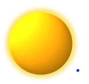
Sodium-like tungsten ions (blue) are far smaller than neutral sodium atoms (orange)—the ion's 11 electrons are pulled in very tightly by the 74 protons in the tungsten nucleus, making their energy jumps far more expensive than in neutral sodium and causing them to emit high-energy ultraviolet wavelengths of light, rather than visible light, as is the case with ordinary sodium. Credit: Talbott, NIST
