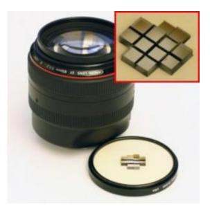
Clustered at the center of an ordinary lens filter are 12 tiny lenses with different focal depths, which project images onto different parts of a camera sensor. Credits - Courtesy Sam Hasinoff
