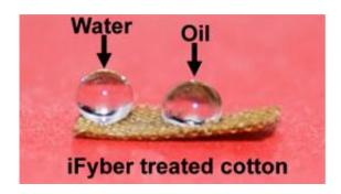
The technology developed at Cornell impart unique properties such as simultaneous water and oil repellency to fabrics while preserving their air permeability and comfort properties.
