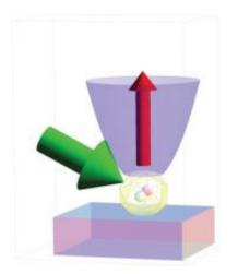
A nitrogen vacancy (small circles) within a diamond crystal shows promise as a "bit" for quantum computers in part because of its great sensitivity to magnetic fields—a sensitivity that also could enable MRI-like studies on objects as small as living cells or single molecules. When green light strikes the nitrogen vacancy, it fluoresces red; detecting variations in this fluorescence permit scientists to extract its information. Credit: J. Taylor, NIST
