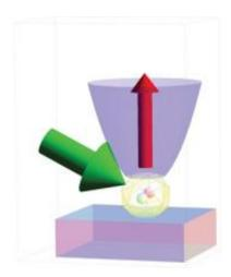
A nitrogen vacancy (small circles) within a diamond crystal shows promise as a "bit" for quantum computers in part because of its great sensitivity to magnetic fields—a sensitivity that also could enable MRI-like studies on objects as small as living cells or single molecules. When green light strikes the nitrogen vacancy, it fluoresces red; detecting variations in this fluorescence permit scientists to extract its information. Credit: J. Taylor, NIST
