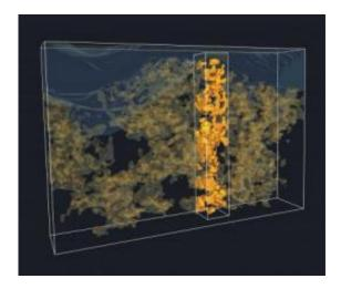
This is a 3-D electron tomography image of a polymer-metal oxide solar cell. The 3-D nanoscopic morphology shows the interpenetrating metal oxide network in (yellow) below an aluminum contact (gray) inside a polymer matrix (black). Credit: Eindhoven University of Technology
