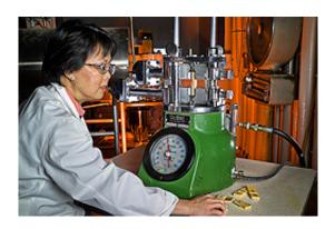
ARS chemist Milagros Hojilla-Evangelista has found a way to make a high-value glue extender for plywood production out of corn germ, a byproduct left over after the corn oil is removed from corn germ meal. Here she tests the breaking point of plywood laminated with vegetable based glue.
