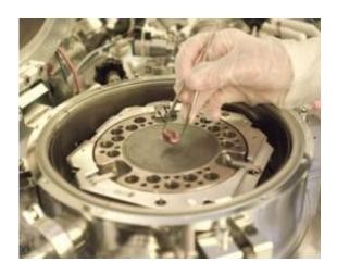
Graduate student Will Chung displays a hybrid chip being developed in Professor Tomas Palacios' lab. The machine in the background is used to combine the semiconductor materials into one chip. Photo - Patrick Gillooly
