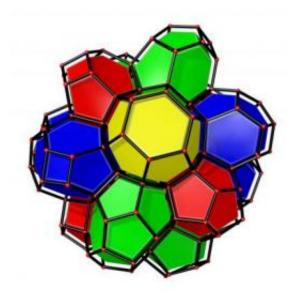
Ruggero Gabbrielli (University of Bath) has developed a new technique for mathematically modeling the structure of foam. He's proposed an alternative solution to the "Kelvin problem.". Whilst the new shape doesn't beat the Weaire-Phelan structure in terms of packing efficiency, the methods he used are a new way of approaching the problem and could ultimately lead to a better solution to the Kelvin problem. Credit: Ruggero Gabbrielli (created using 3dt, part of the Gavrog Project)
