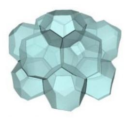
Ruggero Gabbrielli (University of Bath) has developed a new technique for mathematically modeling the structure of foam. He's proposed an alternative solution to the "Kelvin problem." Whilst the new shape doesn't beat the Weaire-Phelan structure in terms of packing efficiency, the methods he used are a new way of approaching the problem and could ultimately lead to a better solution to the Kelvin problem. Credit: Ruggero Gabbrielli (created using Javaview)
