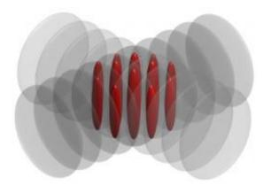
With two laser beams the researchers generate an optical lattice, where the atoms are confined to vertical one-dimensional structures (red) with up to 15 atoms aligned in each tube.
