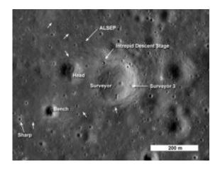
This image from LRO shows the spacecraft's first look at the Apollo 12 landing site. The Intrepid lunar module descent stage, experiment package (ALSEP) and Surveyor 3 spacecraft are all visible. Astronaut footpaths are marked with unlabeled arrows. This image is 824 meters (about 900 yards) wide. The top of the image faces North. Credit: NASA/Goddard Space Flight Center/Arizona State University
