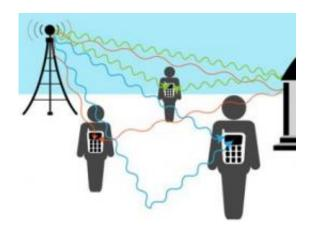
In a wireless network, different transmission frequencies work better for different users. That's because the same transmission reaches each user along several different paths; at one frequency, the signals might reinforce each other, while at another frequency, they might cancel each other out. Photo - Christine Daniloff
