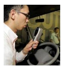
A Toyota Motors engineer blows into a hand-held breathalyser and camera unit during a press preview by Toyota Motors on their breath-alcohol ignition-interlock system in Tokyo, August 31. Toyota said Monday it was developing the anti-drunk driving equipment that would lock the ignition of a vehicle if high levels of alcohol are detected in the driver.
