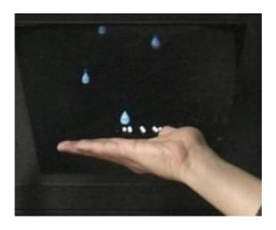
In this demonstration of the touchable hologram, ultrasound is radiated from above and the user feels as if a rain drop hits his palm. Credit: Hiroyuki Shinoda.
