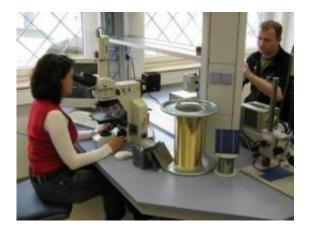
Using a light microscope to study sawed silicon wafer surfaces. In the foreground: a silicon block with sawed wafers, coils of wire and a finished solar cell. Credit: Fraunhofer IWM
