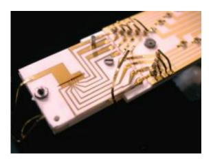
NIST physicists demonstrated sustained, reliable quantum information processing in the ion trap at the left center of this photograph, improving prospects for building a practical quantum computer. The ions are trapped inside the dark slit (3.5mm long and 200 micrometers wide) between the gold-covered alumina wafers. By changing the voltages applied to each of the gold electrodes, scientists can move the ions between the six zones of the trap. Credit: J. Jost/NIST
