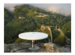
This is an antenna for receiving GPS signals in a geodesy network located in northern Italy. Credit: Copyright 2006 Sigrun Hreinsdottir
