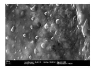
The nano-capsules in the electroplated layer contain a fluid. If the layer is scratched, the layers burst, the fluid escapes and repairs the scratch. Credit: Fraunhofer IPA
