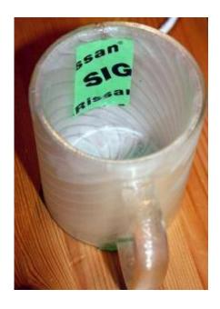
The PCM absorbs the warmth of the mug's content, stores it and brings it down to the optimal temperature. Then the PCM helps maintain the content's temperature at this optimal level by slowly releasing the stored heat back into the mug's contents. Image credit: Fraunhofer IBP.
