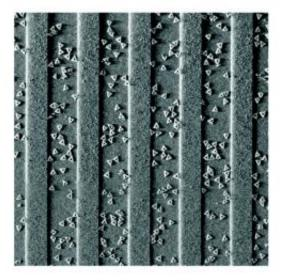
IBM scientists are using DNA origami to build tiny circuit boards; in this image, low concentrations of triangular DNA origami are binding to wide lines on a lithographically patterned surface. Image: IBM
