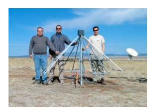
Standing next to a prototype of one of the anticipated 13,000 Long Wavelength Array dipole antennas are (left to right) Brian Hicks, Jake Hartman, and Paul Ray of the NRL engineering team who are installing the latest generation NRL-designed LWA antennas in New Mexico. One of the 27 25-m parabolic dish antennas comprising NRAO's Very Large Array radio telescope appears in the background. Credit: Naval Research Laboratory
