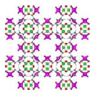
This closeup image of the HKUST-1 metal-organic framework (MOF), recently obtained by NIST scientists, reveals that copper atoms (green) are exposed to the open air within the MOF's lattice-like structure. The exposed copper allows the MOF to safely store acetylene (magenta) up to 100 times more densely than current methods. Credit: Liu, NIST
