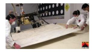
A test setup at NASA's Jet Propulsion Laboratory enables experiments with maneuvers being considered for use by NASA's Mars Exploration Rover Spirit to get Spirit out of soft soil where it has become embedded.
